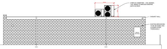
It is proposed that the single air conditioning unit on the roof will be replaced by 1 x double a/c unit and 1x single a/c unit. This is not a like for like replacement. These a/c units are in full public view from all sides of the building and are looked down directly upon by people crossing the footbridge. They are tall and most unsightly as can clearly be seen in the accompanying drawings. It would be preferable that they are sighted elsewhere, possibly at the rear of the building.
